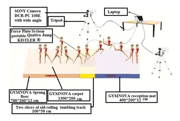
Figure 1. Experimental device.
